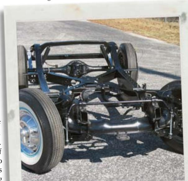
The chassis for the first fuelie, restored as it was when it was specially prepared by Chevrolet's Engineering Center, complete with RPO-581 and waiting for its special fuel-injected engine. But, before we get into that, we've got a special treat for our early fuel injection-loving enthusiasts, next month!
